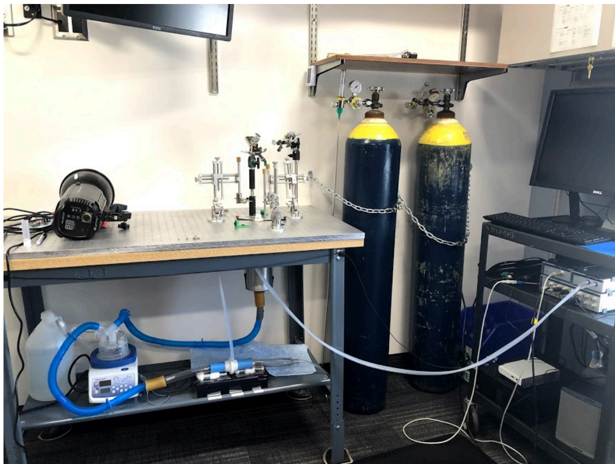
Figure 5. Benchtop setup, humidifier, flow meter, air tanks, and computer system.
