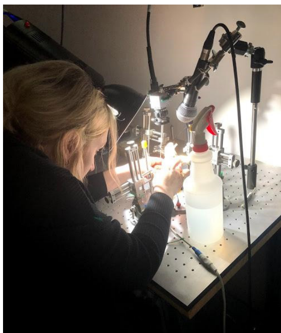
Figure 8. Mounting of pig larynx, with microphone placed superiorly.
